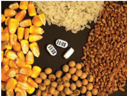
Fig. 1. Tracers for insertion into grain can be marked with an information-carrying code such as a bar code.
