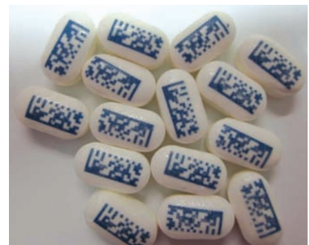
Fig. 3. Two-dimensional data-matrix code printed on tracers.
