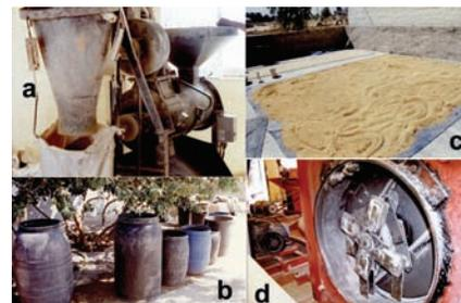
**Fig. 2** Traditional mahangu (pearl millet) milling in northern Namibia. a) PRL type dehuller; b) steeping (lactic acid fermentation) vessels; c) sun drying the fermented grain; and d) hammer mill.
