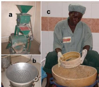
**Fig. 5.** Pearl millet couscous manufactured in Senegal. a) dehuller; b) steamer; and c) agglomerating and sifting the couscous.
