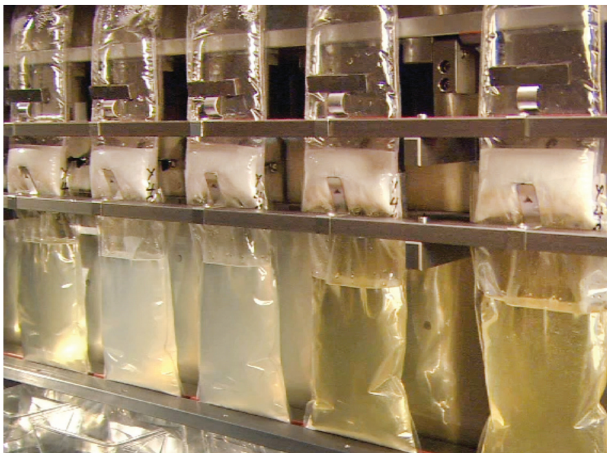
Fig. 2. Transfer of digested sample filtrate into the soluble dietary fiber filter bag for the precipitation phase.
