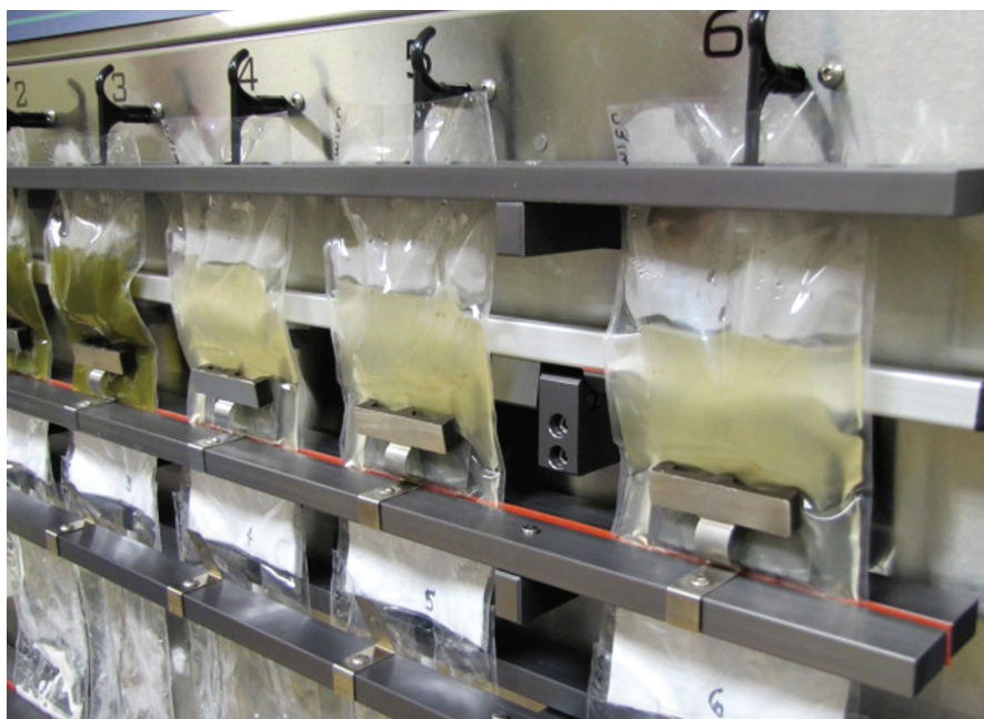
Fig. 1. Dual-compartment insoluble dietary fiber filter bag has an upper chamber for enzyme digestion and a lower section for filtration.
