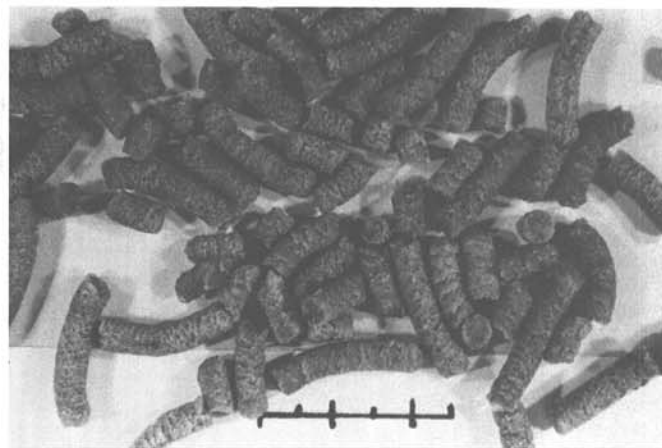
Fig. 1. Sorghum pellets after cold extrusion and cooking (line = 2.5 cm).
