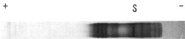
Fig. 10. Slab gel electrophoresis pattern of 13S globulin in the urea system under conditions described for Fig. 4.
