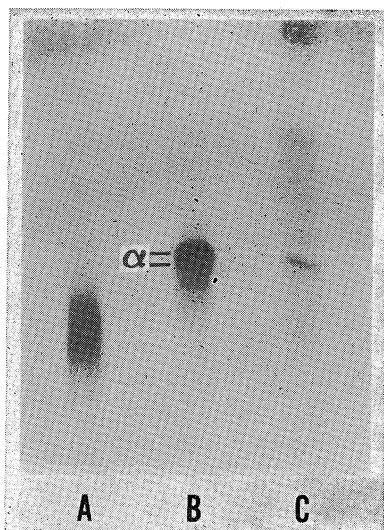
Fig. 6. Starch-gel electrophoresis of alpha-gliadin fractions obtained by gel filtration (Fig. 3) in a buffer of 0.005M aluminum lactate, 0.02M lactic acid, and 3M urea.
