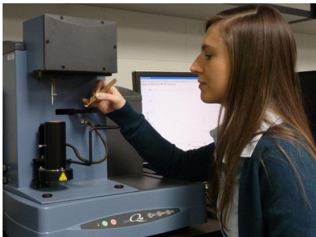
**Figure 1.** Alejandra Billiris setting up a rice kernel for analysis in a thermogravimetric analyzer. The instrument is being used in this research to accurately measure mass loss during drying of the kernel, from which Alejandra can calculate the drying rate.
