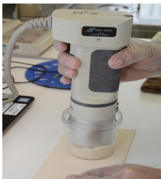
Fig. 5. Minolta Chroma Meter measurement of boiled udon noodle color using an Agrtron cup to compress 60 g of boiled noodles. Source: AEGIC.
