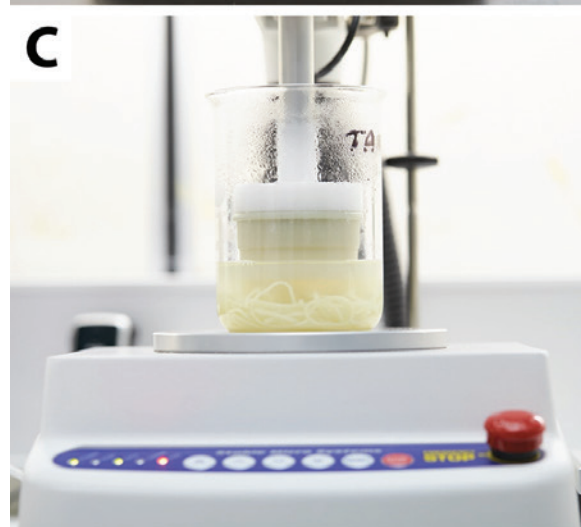
Fig. 6. Measurement of noodle firmness, chewiness, and extensibility using a texture analyzer (Stable MicroSystems). A , A flat probe (1 mm), most commonly used to measure firmness for udon noodle standards; B , tensile strength test measuring the extensibility of boiled noodle strands; C , new triple cutting ring system used to measure firmness of noodle strands with or without soup. Source: AEGIC.
