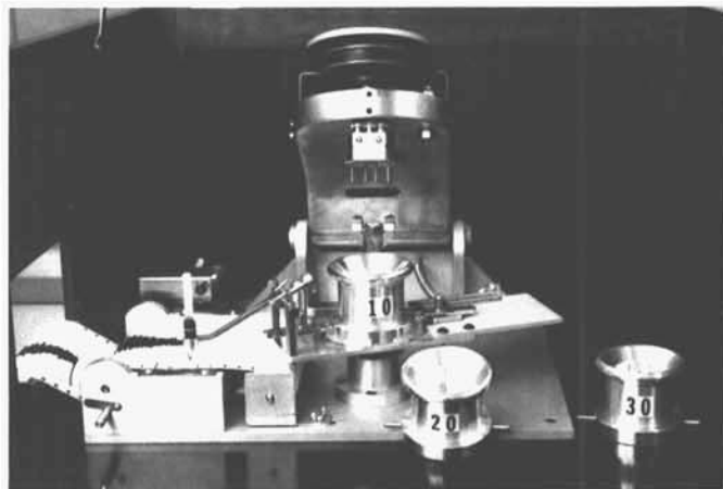
Fig. 1. Mixograph for recording mixing properties of 5-g samples of wheat flours. Bowl no. 10 is in operating position (on the bowl platform) directly below the raised mixing head and its two planetaries. Each planetary has two pins that revolve in a predetermined pattern about three stationary pins in the bowl. Attached to the right side of the bowl platform is the rectangular damping arm. The spring is attached to the back of the mixograph, and its slot hook is attached on the damping arm. To the left of the bowl platform is the balanced pen arm. Screw-in pen with black drawing ink exerts only about 6 g of pressure on the recording paper.
