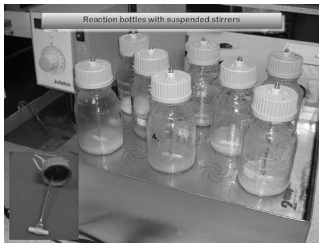
Fig. 3. Picture showing a 2mag Mixdrive 15 submersible magnetic stirrer in a custom made water bath. This allows stirring of 15 samples at controlled speed and 37°C.
