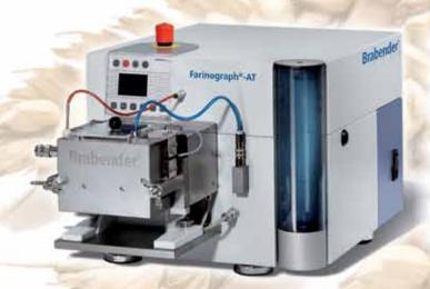
The automatic titration system alleviates operator error and improves accuracy for the entire line of Brabender<sup>®</sup> mixers
