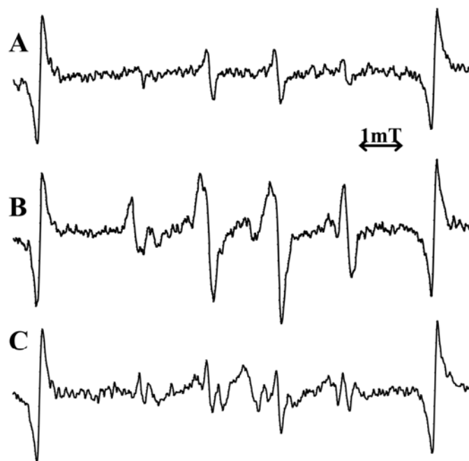
Fig. 6. Detection of S• on SS-reduced GP-1 by DMPO spin-trapping ESR spectroscopy. Solution of 20% SS-reduced GP-1, 1 mmol/L of DTPA, 2 \mu\text{mol/L} of Rf, and 75 mmol/L of DMPO in 25 mmol/L of PIPES buffer, pH 7.0 (SS-reduced GP-1 sample) at room temperature in darkness (A) or in white light at 650,000 lx (B). Trace (C) was recorded under identical conditions as for (B) except using a solution of nonreduced GP-1.
