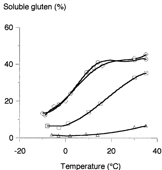
Fig. 2. Gluten sample soluble portion by mass-recovered method 60 ( \circ ), 70 ( \diamond ), 80 ( \square ), and 90 ( \Delta ) (v/v) ethanol solutions using a 20:1 solvent-to-sample dilution.
