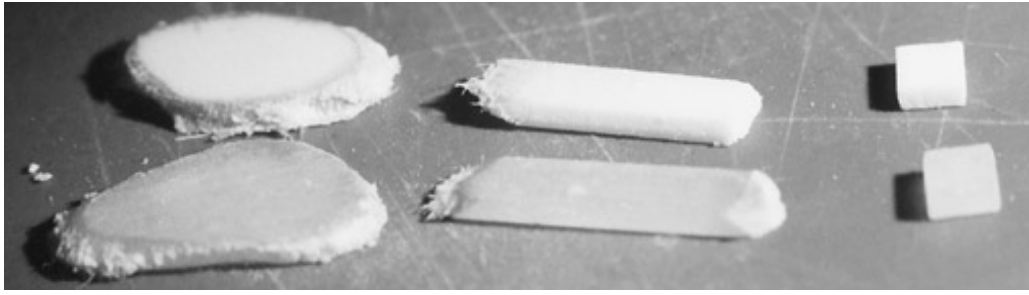
Fig. 4. Steps 2–4 (Fig. 1). Manufacture of test samples of mealy and vitreous endosperm: after step 2 (left), after step 3 (center), after step 4 (right).
