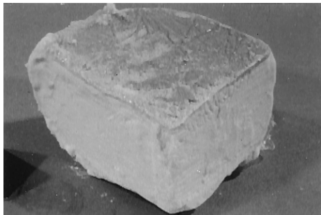
Fig. 2. Centrifugally separated wrinkled pea starch from the underflow of the hydrocyclones used for starch refining. Protein layer content = 1.5% dry matter.
