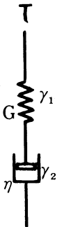
Fig. 4. A simplified model for gas cells in dough and equations for internal (p) and overall (P) pressures.
