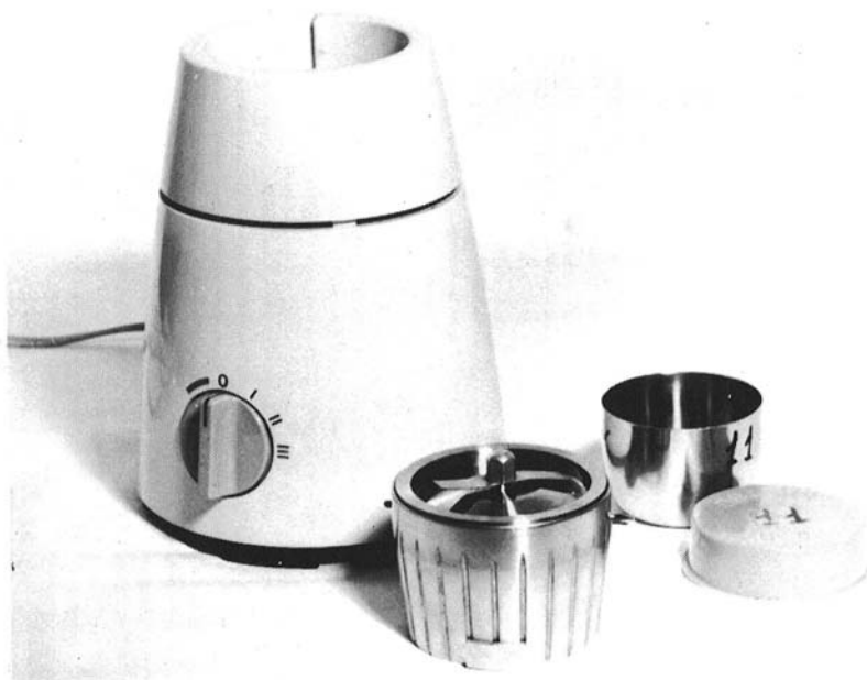
Fig. 1. Laboratory grinder used in the FHI-method. (Manufactured by Holm & Halby, Egegårdsvej 5, 2610 Rødovre, Copenhagen, Denmark.)
