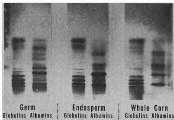
Fig. 2. Starch-gel electrophoretic patterns of albumin and globulin proteins separated from 0.5M NaCl extracts of corn grain, endosperm, and germ. Origin is at bottom of gel. Direction of migration is upward to negative electrode.
